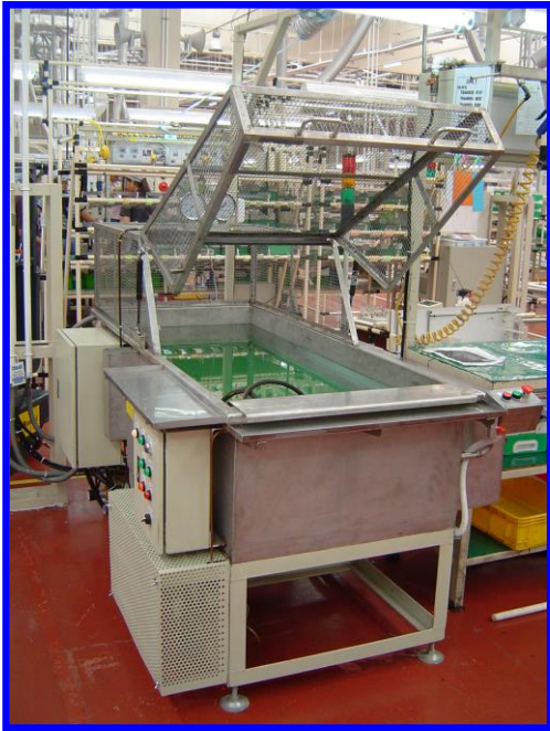
35BAR LEAK CHECK
