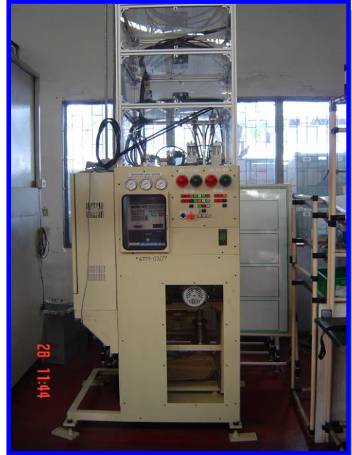
PRESSURE & VACUUM TEST
