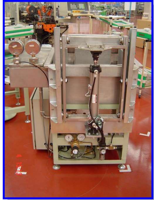
35BAR LEAK TEST
