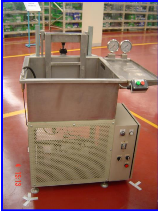
35BAR LEAK TEST
