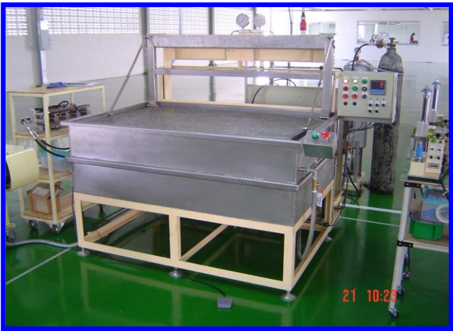
3.5 MPa LEAK TEST
